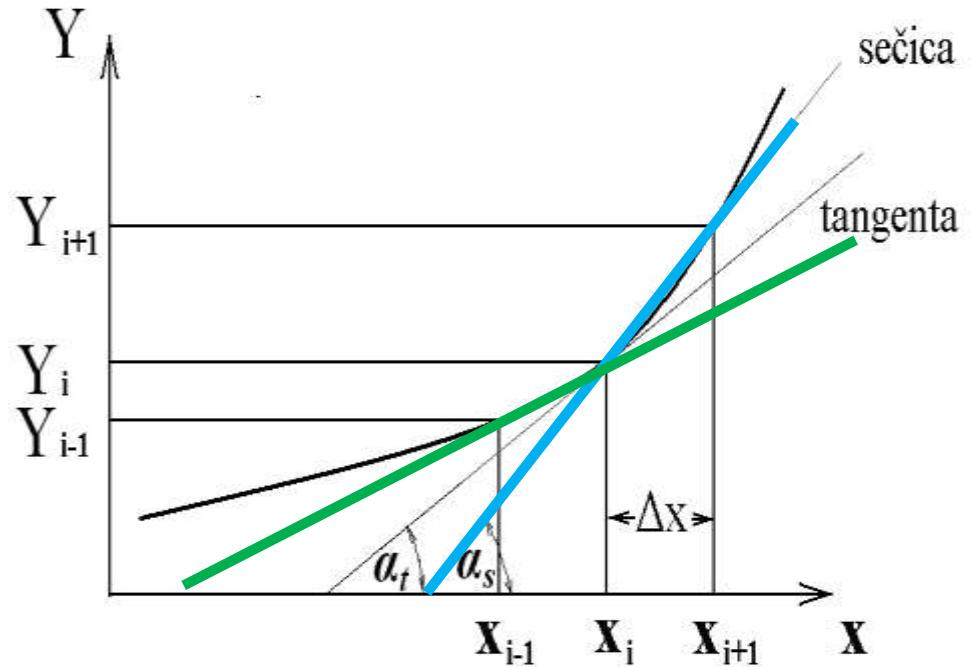
$$\left. \frac{\partial^2 Y}{\partial x^2} \right|_x \approx \frac{\frac{\partial Y}{\partial x} \Big|_{x + \Delta x / 2} - \frac{\partial Y}{\partial x} \Big|_{x - \Delta x / 2}}{\Delta x} = \frac{\frac{Y_{i+1} - Y_i}{\Delta x} - \frac{Y_i - Y_{i-1}}{\Delta x}}{\Delta x} = \frac{Y_{i+1} - 2Y_i + Y_{i-1}}{\Delta x^2}$$
