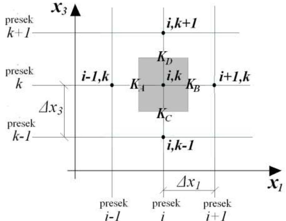
$$\frac{K_B \frac{\Pi_{i+1,k} - \Pi_{i,k}}{\Delta x_1} - K_A \frac{\Pi_{i,k} - \Pi_{i-1,k}}{\Delta x_1}}{\Delta x_1} + \frac{K_D \frac{\Pi_{i,k+1} - \Pi_{i,k}}{\Delta x_3} - K_C \frac{\Pi_{i,k} - \Pi_{i,k-1}}{\Delta x_3}}{\Delta x_3} = 0$$
